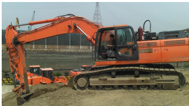
Figure 8: PRB installed 38ton excavator testing, Doosan's DX380LC-3
