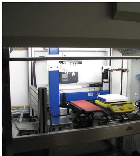
**Figure 5.2:** Automatic dip-coating machine placed in a bio-flowbox.
