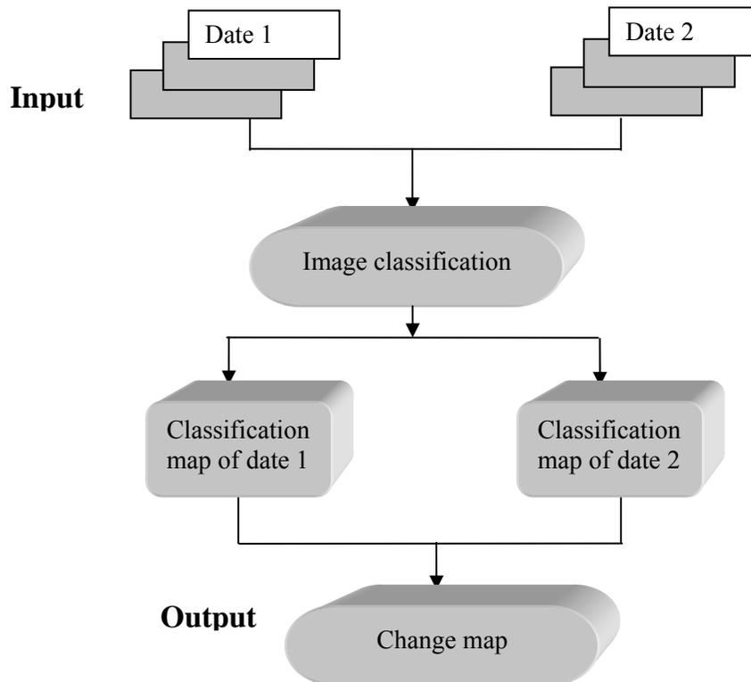
Figure 3.4 A flowchart of post-classification change detection technique
