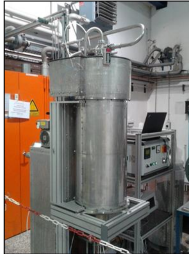
Figure 92: Reetz vertical tube furnace 1650 to adjust oxidation state.
