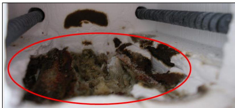
Figure 91: Damages caused by slag boil over within a high temperature furnace.
