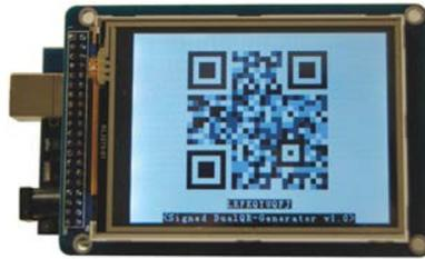
Figure 1: Arduino Prototype With LCD Display Attached
