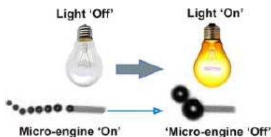
Scheme 7.1: New method of microjet control by a white light source is shown. Optical microscopy images (bottom) show individual self-propelled (left) and stopped (right) microengine right after it was illuminated using a white light source.
